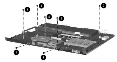
Removing the System Board Screws
